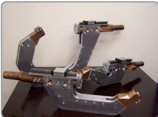
Modular robot gun arms with linear slides made from both high strength aluminium and CuCrZr.
