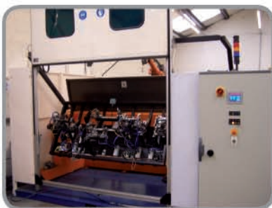
Mig welding robot cell with orbital turntable for welding fascia assemblies
