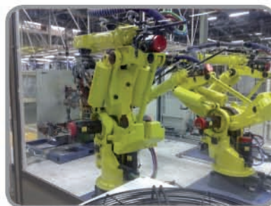
Triple robot cell for welding rear quarter bodyside assemblies
