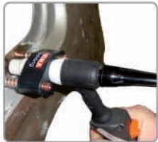
Single sided spot tig tool DRT, with fast earth system DRMT
