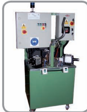
3 Headed spot welder for welding fuel hose necks
