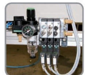
Pneumatic unit with filter and self-governing relay.
