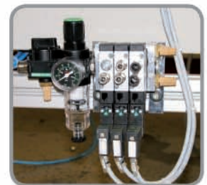
Pneumatic unit with filter and self-governing relay.
