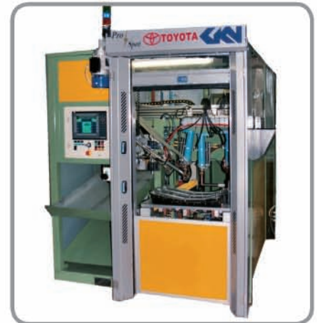
3 Headed multi projection welder with eject station
