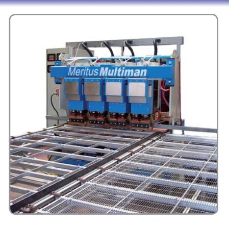
A modular resistance welding system developed for medium to high volume production of flat or profiled panels using pre-cut length wire.
