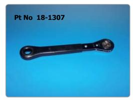
Manual tip dresser 18-1307 can quickly remove the mushroomed portions of the electrodes and renews the operating contour. The dresser machines both upper and lower electrodes "on the job". The dresser is 250mm long with a replaceable hardened tool steel cutter (18-130701) Cuts 5mm dia x 120 angle
