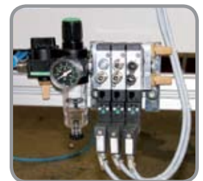
Pneumatic unit with filter and self-governing relay.
