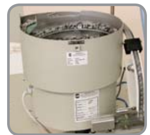
The hopper has a capacity of 3,5 litres. Nut movement by vibration.
